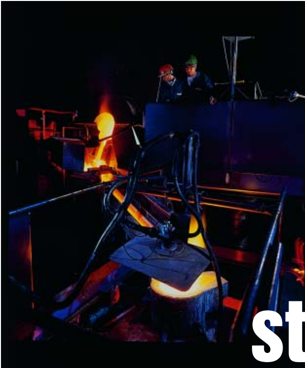
The final stages of silver refining at Hoboken. Gold is the other main precious metal recovered from copper anode slimes
